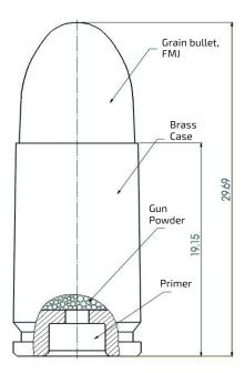
Image: Components Layout (9 x 19 mm NATO BALL FMJ 7.5 g (115 gr)) Part number: 9101907
